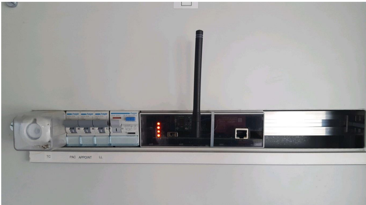
Figure 43 - Picture of the first prototype version of the gateway installed in the electrical cabinet.
